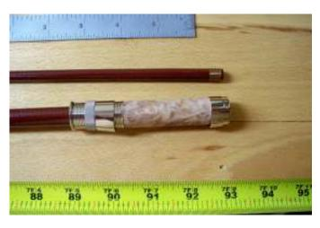
5) Once everything is checked and double checked, you can epoxy the dowel into the blank and then epoxy the seat as usual.
