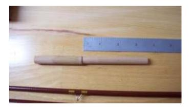
3) Now you have to make an insert that you can turn down to accept the seat insert. Best material to use is a wooden dowel that is either the same diameter as the ID of the blank or slightly oversize. Put a slight taper so it will slide into the blank a few inches. Three inches into the blank would be great, but there is no hard and fast rule. Next, you want to turn the diameter of the dowel down until the reel seat insert will slide over the dowel. See note below on turning the dowel down.
