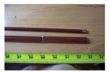
2) Next, you have to cut off the assembled seat length from the butt end of your blank.
