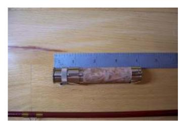
Measure the overall length of you reel seat, with it assembled, from the butt cap to where it will contact the blank.
