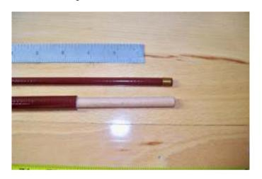
4) Dry assemble everything to ensure that everything fits snug. Not so snug that the parts fitting up will act like squeegee and remove all the epoxy off as the parts are assembled. During the dry fit up check to ensure the blank is the proper length with the seat installed.
